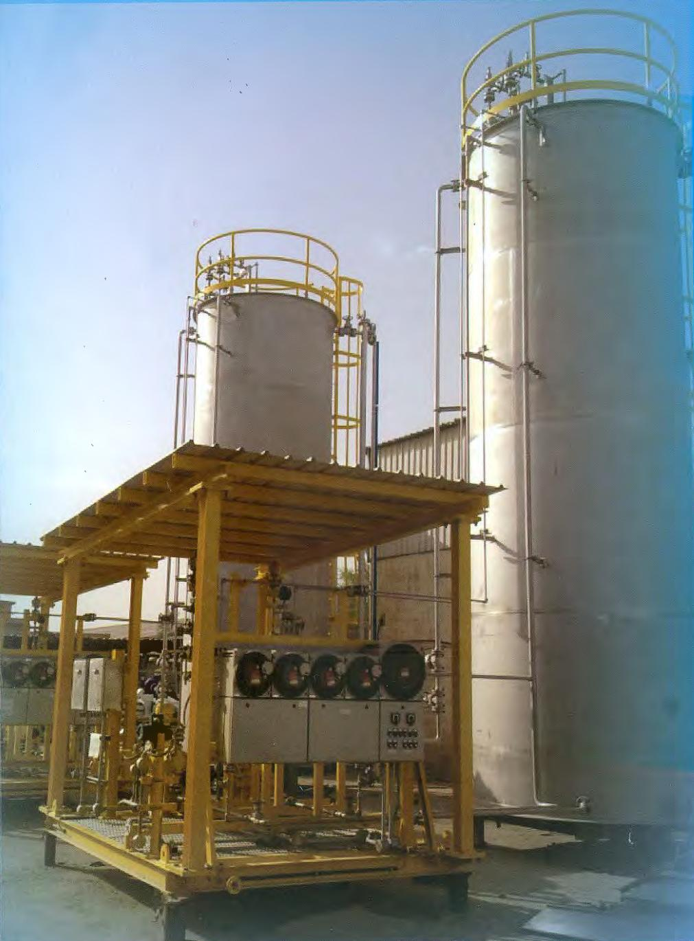
TANK store the chemicals which need to be injected into the process or systems. The tanks usually are either of horizontal cylindrical having dished end or vertical cylindrical with flat/conical/ dished bottom and flat/dished top or of rectangular construction. The applicable design codes can be as per the ASME Sec VIII U-stamped, API 650, UL 142, BS 2654, BS 4994. The material of construction can be CS, SS304, SS316, SS316L or GRP. Tanks can be coated as per the client's requirement.
